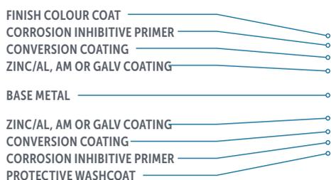
NOTE: CUT EDGES ARE CATHODICALLY PROTECTED BY GALV OR ZINC/AL COAT WHICH INHIBITS THE BASE METAL RUSTING.
